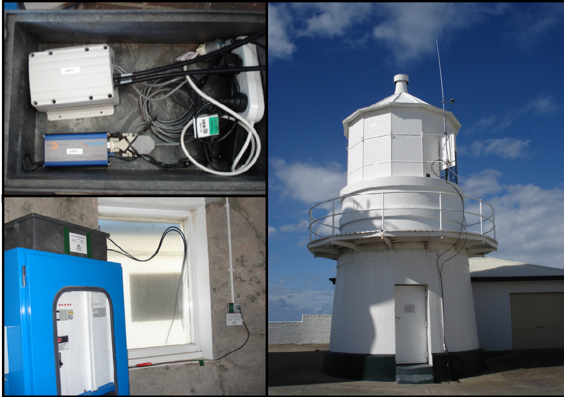
Figure 2: AIS Trial 1 setup at Nobby's Head Lighthouse, showing the equipment crate (top left), the location of the crate on the lower floor (bottom left), and the positioning of the VHF and GPS antennae on the exterior (right).
